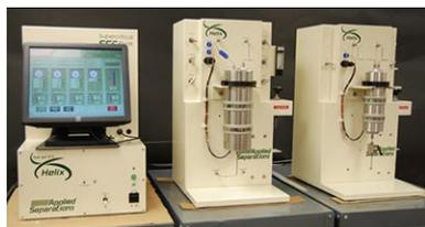
SFE is an alternative extraction technology that uses supercritical CO<sub>2</sub> to recover trace analytes from
